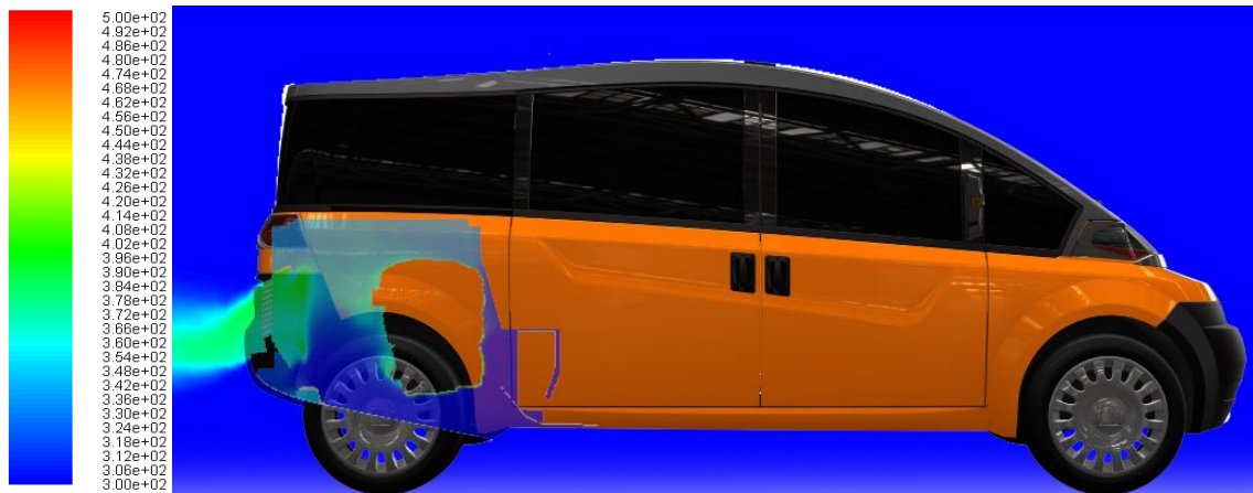
Temperature contours (K) of cooling analysis results of combined engine and radiator compartments
