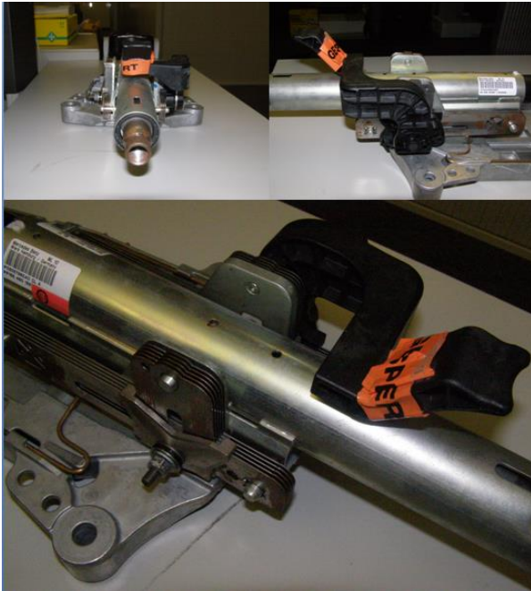
Figure 7. Spring Type Clamp Lever Mechanism
