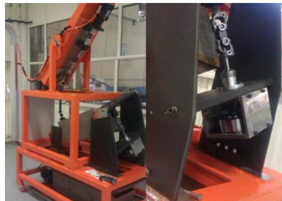
Figure 20. Torque to Rotate & Torsional Endurance with Mud Water Test Bench
