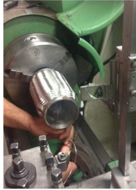
Figure 4: Radial stiffness measurement for flex-pipe.
