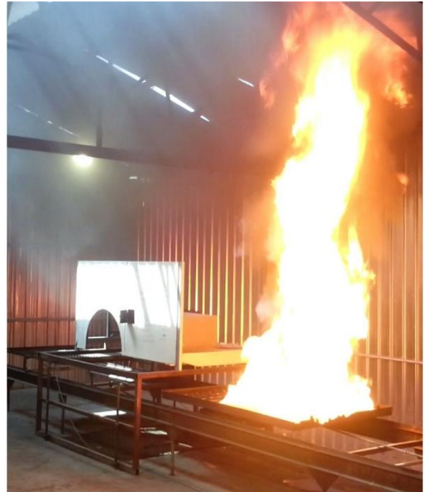
Figure 8 – Moving the preheated pan under the fixture
