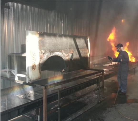
Figure 10 – Fuel Tank After Fire Test
