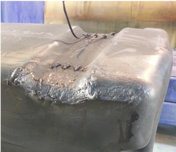
Figure 11 – Fuel Tank After Fire Test
