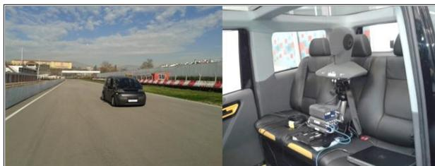
Figure 5. Test at the track and the artificial head in rear seat of the vehicle.
