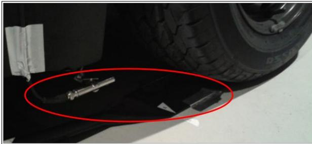
Figure 4. Tire patch placement example at test in semi-anechoic chamber.
