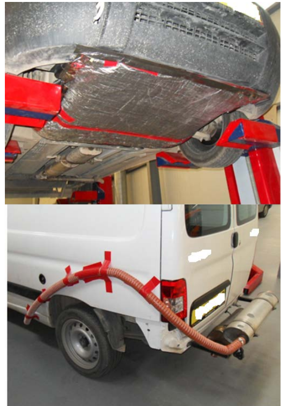
Figure 2: The Applications of Undershield and Total Exhaust Muffler
