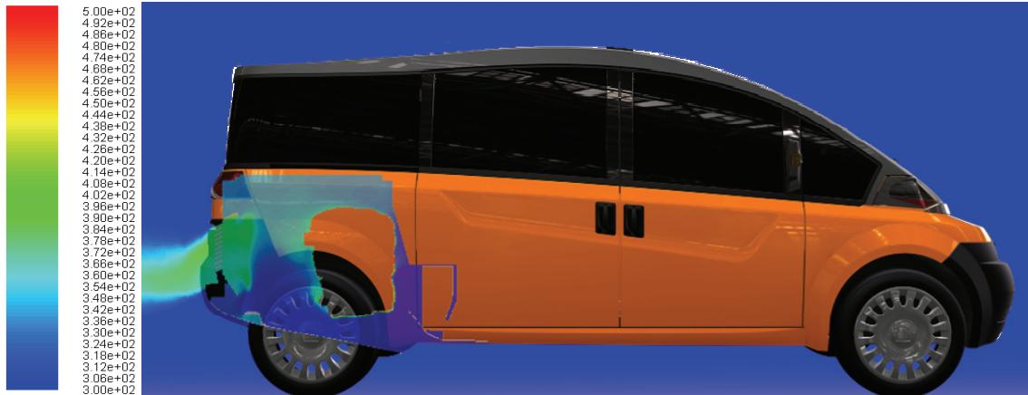
**Figure 5 Temperature contours (K) of cooling analysis results of combined engine and radiator compartments**
