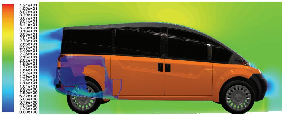
**Figure 6 Velocity contours (km/h) (no level difference between base level of the vehicle and engine compartment intake) (Velocity: 25km/h)**
